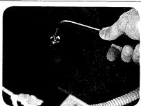
Surface probes Use these to check the temperature of flat cooking equipment, such as griddles.
