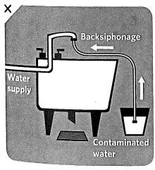
Backflow prevention The best way to prevent backflow is to avoid creating a cross-connection. Do NOT attach a hose to a faucet unless a backflow prevention device is attached. A vacuum breaker is a mechanical device that prevents backsiphonage. It does this by closing a check valve and sealing the water supply line shut when water flow is stopped.
