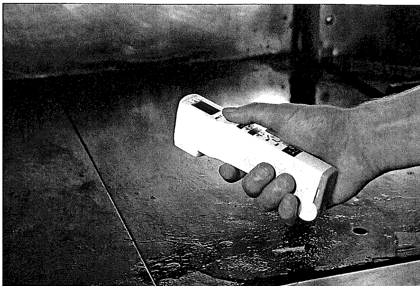
Figure 2.23: Infrared thermometers measure the temperatures of both food and equipment.
